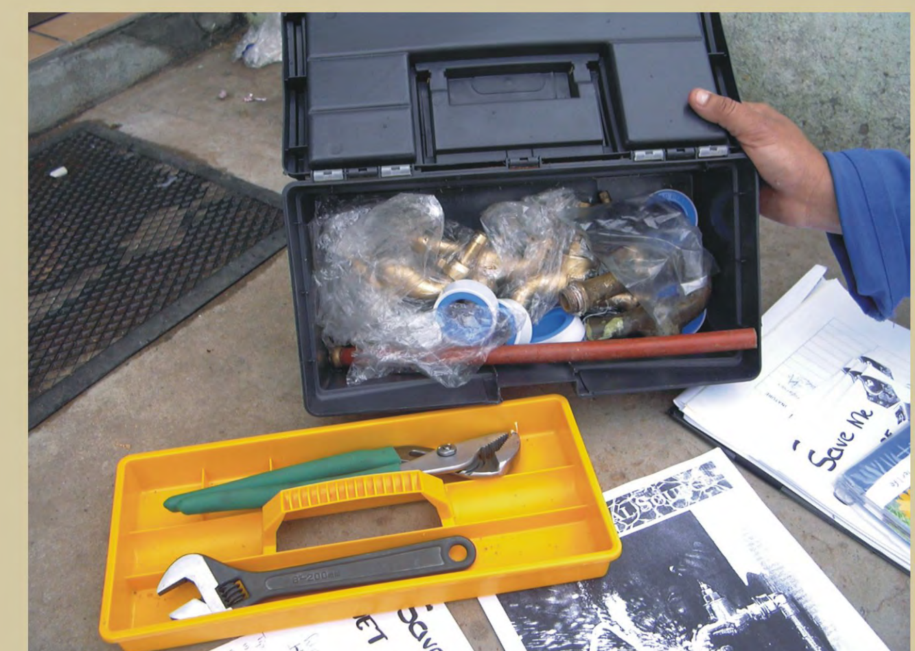
Figure 6. Complete leak repair kits were purchased and supplied to the repair teams,
